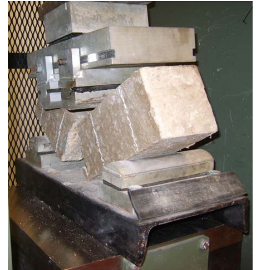
Concrete beam failure
