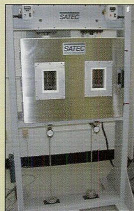
The experimental setup for long-term room temperature testing of 12 liners (left) and one of the loading frames and environmental chambers for creep-deformation testing.
