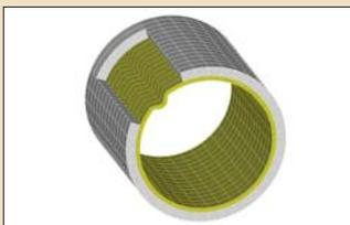
(Figure 1) 3-D FE model of a fully deteriorated lined cast-iron pipe.
