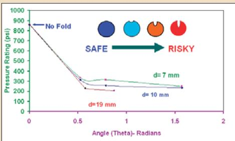
(Figure 3) Pressure rating of CIPP liner bridging a gap in the host pipe as a function of the geometry and size of the longitudinal fold.
