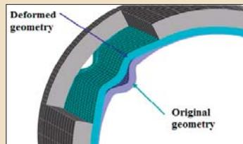
(Figure 2) Initial and final geometries of a longitudinal fold in a GRF CIPP liner subjected to internal pressure.
