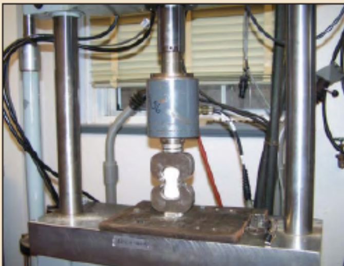
Fig 1. Tensile testing of a fiber-reinforced briquette
