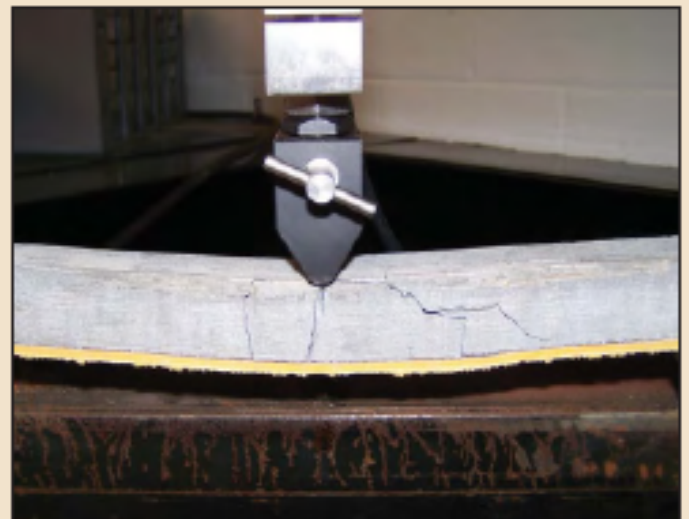
Fig 2. 3-Point Bending test of a grout-fiber-liner specimen
