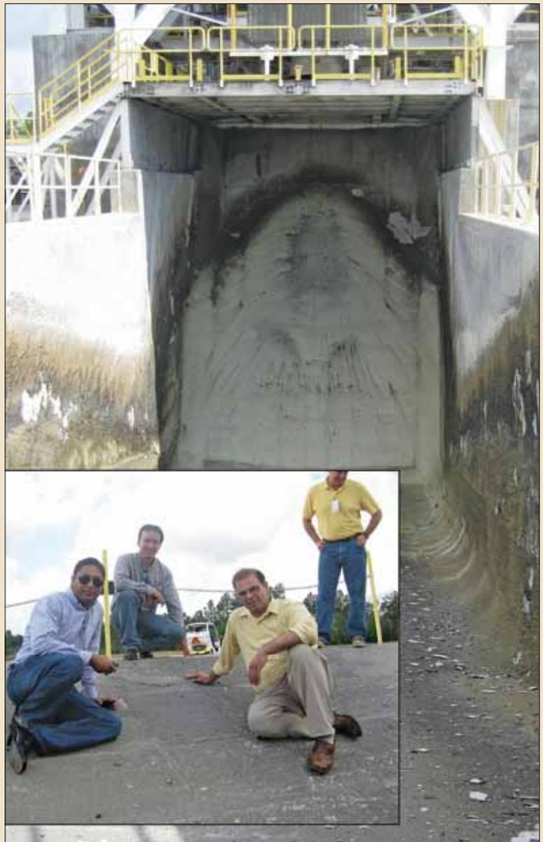
Drs. Allouche, Montes, and Kupwade-Patil inspecting a test patch of Geopolymer concrete in the flame trench following an AJ 26 rocket engine test in NASA’s Stennis Space Center. In view of the product’s successful performance, a comprehensive testing of the TTC’s HTGeopolymer product line is scheduled to take place at Stennis later this summer.
