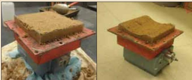
Figure 1: Plexiglass guide (left) and shaped soil surface (right)
