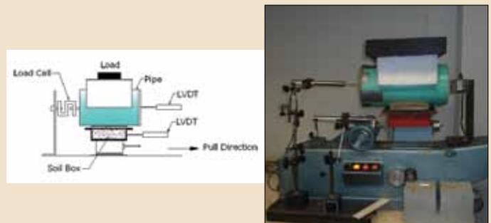
Figure 2: Second set-up – schematic (left) and actual (right)
