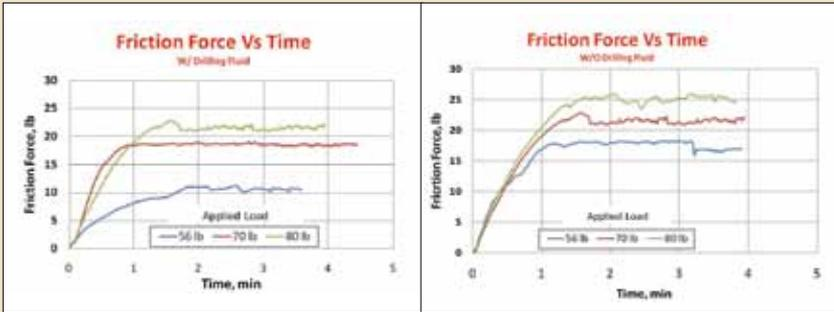
Figure 3: Friction Force between 8 in. pipe and sandy soil with (left) and without drilling fluid (right)
