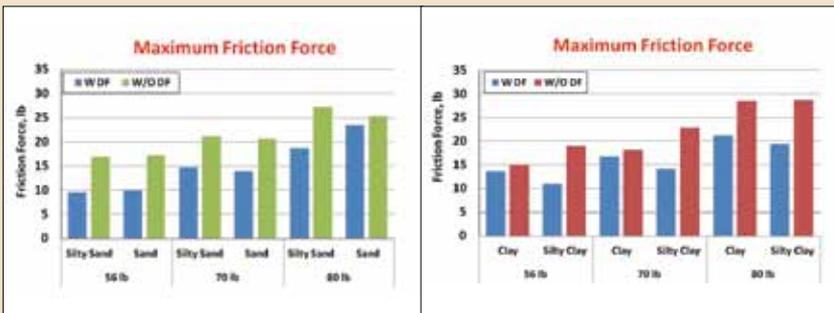
Figure 4: Friction Force between 8-in. pipe with sandy soil (left) and with clay soil (right)
