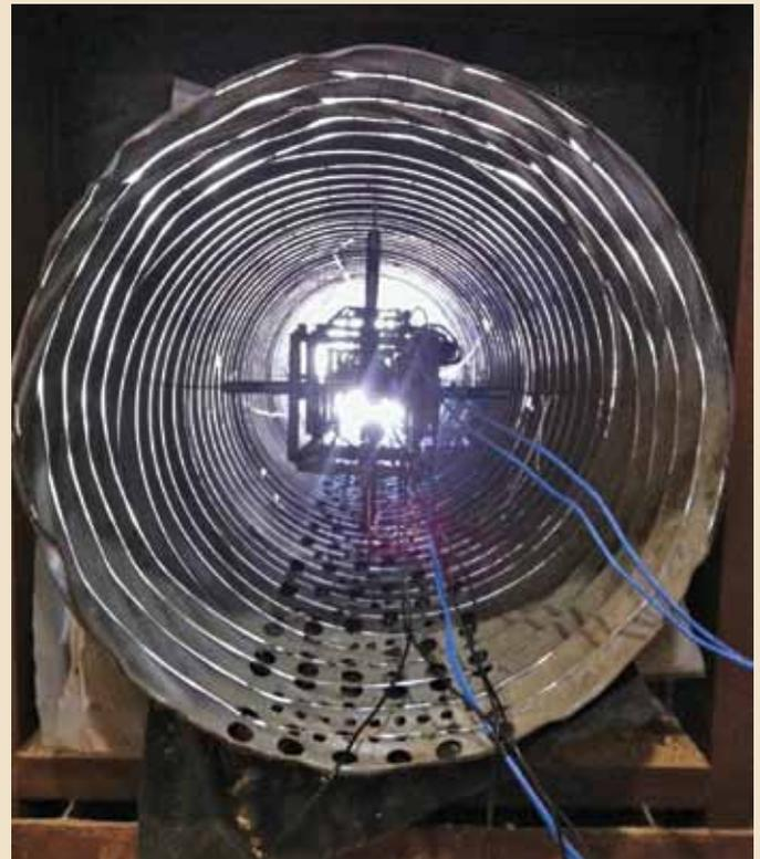
This research uses either exhumed deteriorated corrugated metal pipe culverts or corrugated metal pipes which were deteriorated by mechanically removing 25 percent of the metal within a pre-determined arc along the lower half of the culvert.
