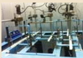
Inside environmental chamber: long-term creep rupture testing. (tensile creep testing shown)
