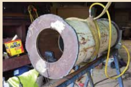
Burst pressure testing of specimens with installed internal seals.
