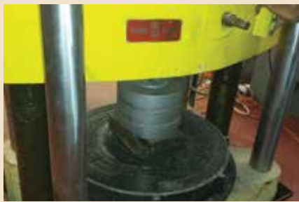
Manhole cover under testing in vertical actuator.
