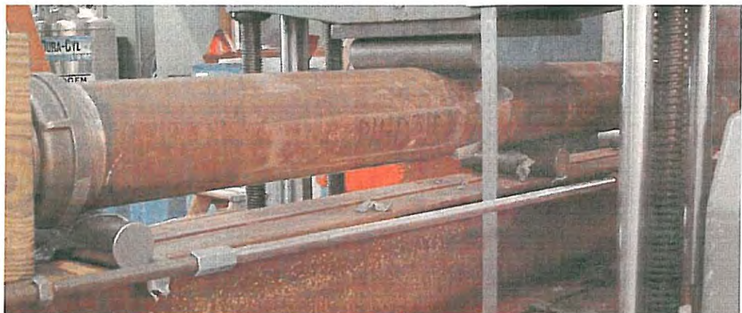
Figure 1: Sample PII-DJIP-3 in the UTM fixtured for shear deflection testing of the butt joint (behind vertical scale).
