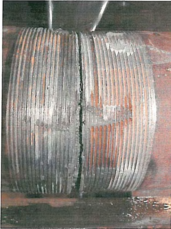
Figure 2: Sample PII-DJIP-4 at 0.49 inches deflection (with leakage).
