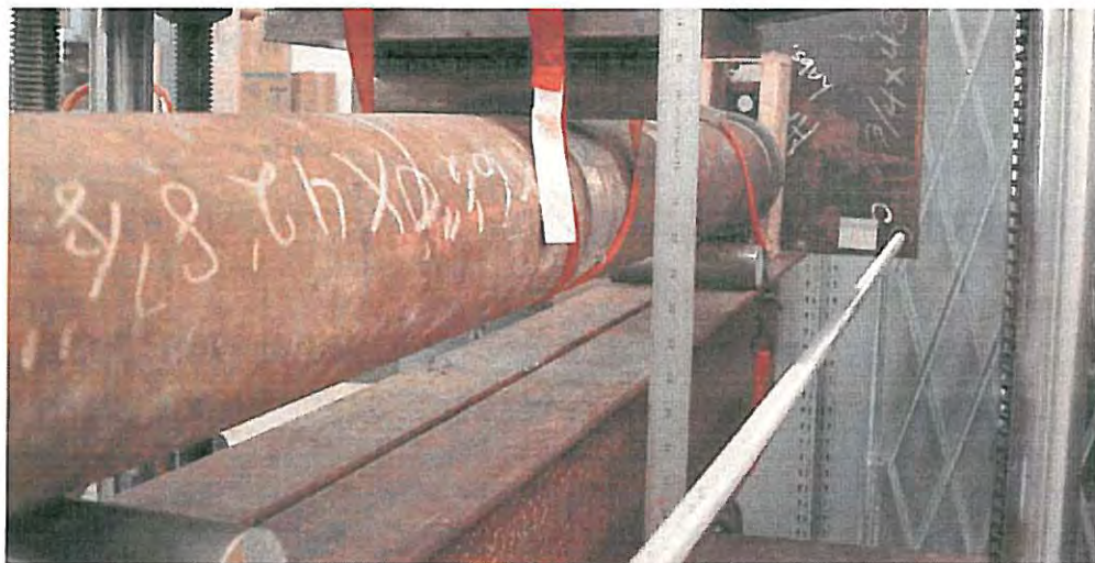
Figure 1: Sample PII-DJIP-4 in the UTM fixtured for three-point bend testing of the butt joint (just left of the vertical scale).
