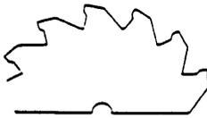
FLOORING BLADES are tungsten carbide-tipped blades especially designed for rough cutting where occasional nails, metal lathe, etc. will be cut. It is especially recommended for the professional carpenter or installer of air conditioning or heating ducts where it is necessary to cut through old walls and floors. Always wear safety goggles when cutting metal.
